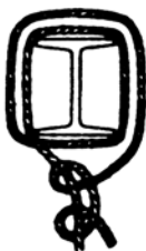
Bad Practice Steel can cut rope
